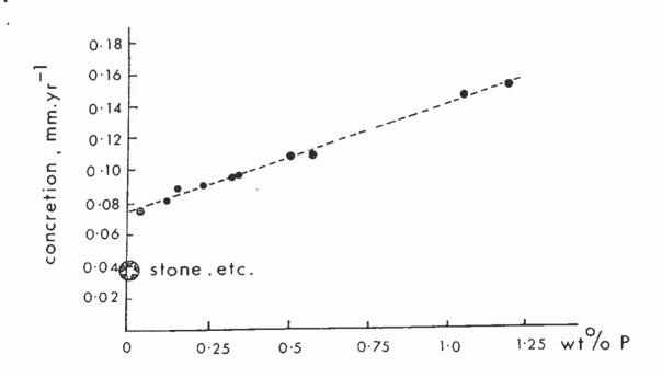
Fig. 1: Effect of phosphorus on the rate of concretion formation on marine growth.
